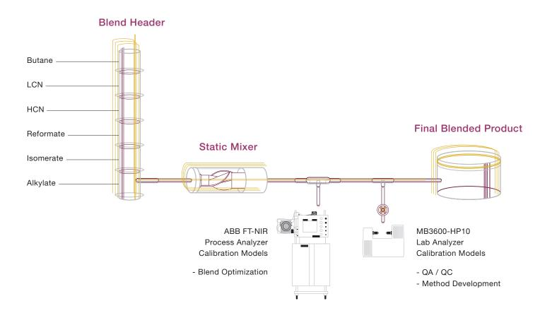
The MB3600-HP10 laboratory analyzer is designed and configured for routine hydrocarbon analysis and for easy calibration modelling and method preparation. It includes all the hardware, software and accessories required for both QA/QC analysis and chemometrics development.
