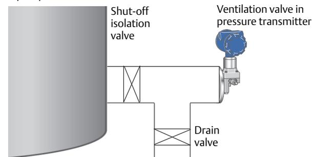
Shut-off isolation and drain valves used for zero calibration of the pressure transmitter.
