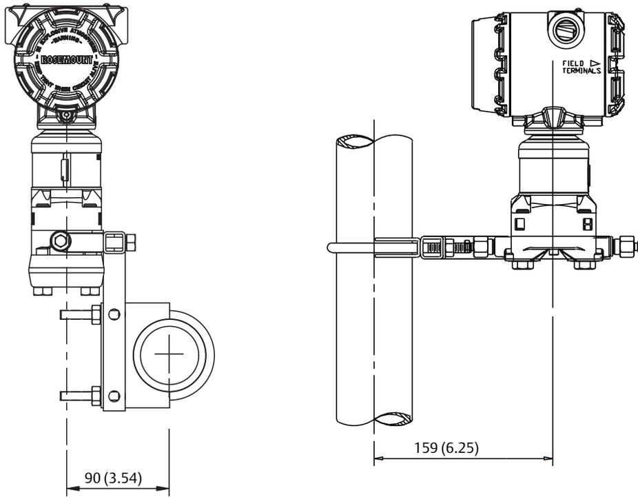
Figure 4. Panel installation
