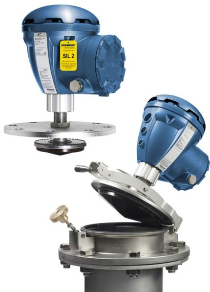
The Rosemount 5900C with array antenna is a non-contact radar level gauge for still-pipe measurement. It is available in two versions, Fixed and Hinged Hatch. Typical applications are crude oil tanks with floating roofs and gasoline/product tanks with or without inner floating roofs.
