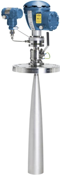
The Rosemount 5900C with LPG/LNG antenna is a non-contact radar level gauge for measurement on pressurized or cryogenic liquefied gas. Radar signals are transmitted inside the still-pipe which enables the gauge to have a sufficiently strong echo even under surface boiling conditions.
